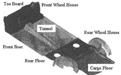
Figure 2 - Areas where damping treatments are applied.
