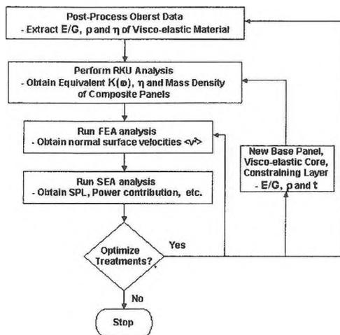
Figure 1 – FEA/SEA Modeling & Design Iteration Process.
