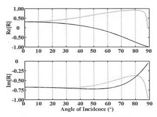
Fig. 2. Angle dependence of the real and imaginary parts of the reflection coefficient R of a suspended acoustical ceiling, at 63 Hz: Extended reaction - grey line; Local reaction – black line.
