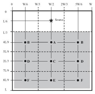
*Figure 1. Diagram of a generic classroom, showing the generic source and received positions, with coordinates.*
