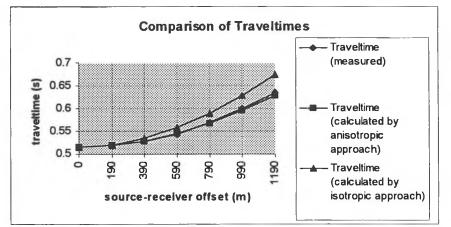
Comparison of measured and calculated traveltimes for a laboratory experiment involving a transmission of acoustic signal across a two-layer anisotropic medium separated by a planar interface. The source-receiver offset corresponds to the separation measured parallel to the interface. The actual dimensions of the physical sample used have been scaled to allow data processing using software developed for seismological studies.
