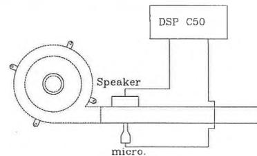
Figure 2 Scheme of the developed control system
