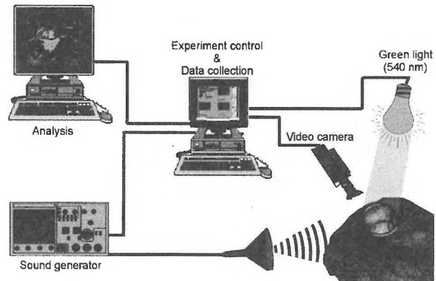
Fig. 1 Experimental setup for recording intrinsic signals
