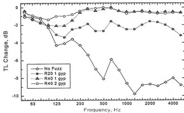
Figure 3. Effects of roof vents on RHWT roof.
