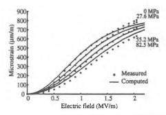
Fig. 2. Strain versus electric field at various prestresses
