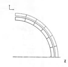
Fig. 6. Strained structure of the PMN spherical shell submitted to an initial voltage and a voltage step. Full line: strained structure, dashed line: initial structure
