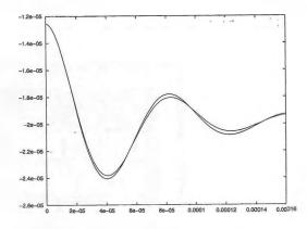
Fig. 5. Displacement of the PMN shell submitted to 1000 V step (initial voltage of 4000 V) versus time. Thick line: semianalytical model (LC), thin line: finite element model (FE)
