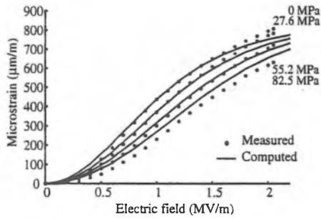
Fig. 2. Strain versus electric field at various prestresses
