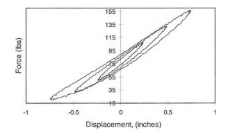
Fig. 1: Dynamic force-deflection of a seat cushion under different excitation amplitudes at 1.5 Hz.
