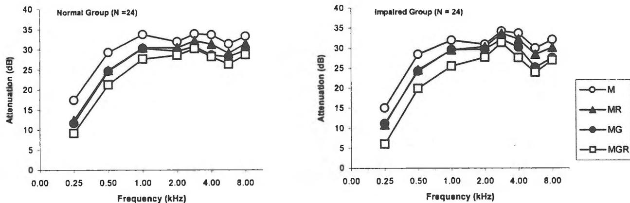
Figure 1. Attenuation as a function of frequency. Effects of ear condition and hearing status.
