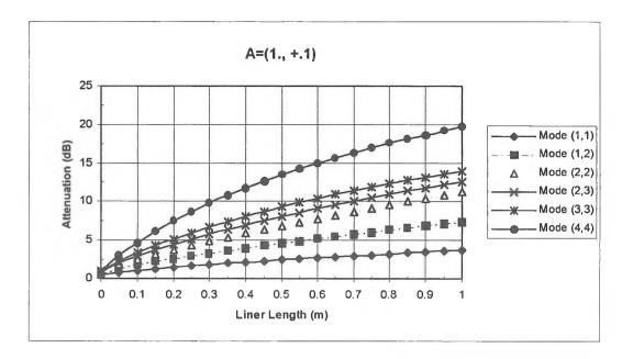
Figure 7: Modal attenuation  $(\Pi_t^{II}/\Pi_i)$  as function of liner length for different incidents modes and a normalized acoustic admittance A = (1., +.1)
