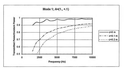
Figure 3: Total transmitted to incident power ratio  $(\Pi_t^{II}/\Pi_{m0})$  as function of frequency for incident mode 1 and a normalized acoustic admittance A = (1, +, 1)
