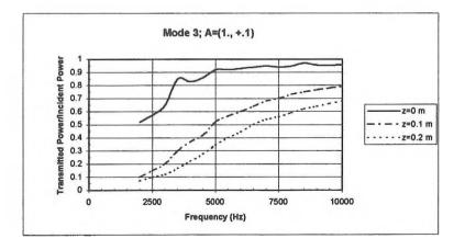
Figure 4: Total transmitted to incident power ratio  $(\Pi_t^{II}/\Pi_{m0})$  as function of frequency for incident mode 3 and a normalized acoustic admittance A = (1, +, 1)
