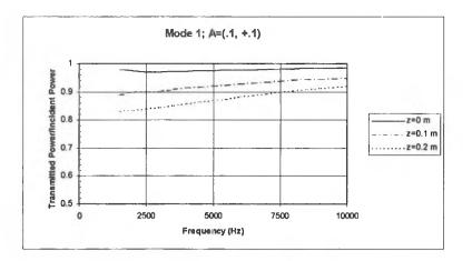
Figure 2: Total transmitted to incident power ratio  $(\Pi_t^{II}/\Pi_{m0})$  as function of frequency for incident mode 1 and a normalized acoustic admittance A = (.1, +.1)
