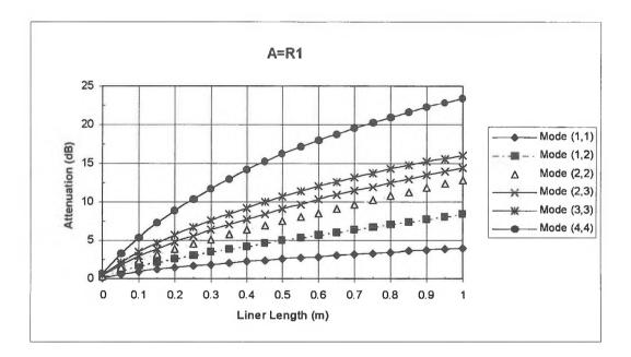
Figure 8: Modal attenuation  $(\Pi_t^{II}/\Pi_i)$  in function of the distance for different incidents modes and a normalized acoustic admittance A = R1
