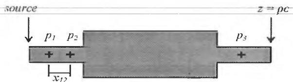
Figure 2. Measurement Locations for 3-Point TL Formulation
