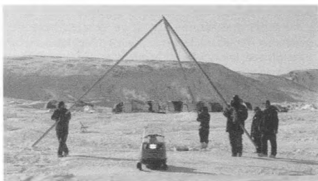
Fig. 2. A tripod is setup to support the weight of an ice drill; the ice camp is in the background.
