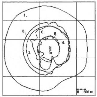
Figure 3: Modelling results, calm winds, 50 dBA contours shown. Each square is 1 km by 1 km. *1*. Basic modelling; 2. Basic modelling with atmospheric attenuation; 3. ISO-9613, ground attenuation G=0; 4. ISO-9613, with G=1; 5. ISO-9613, G=1, complex terrain; 6. ENM with soft ground, calm winds and E stability class.
