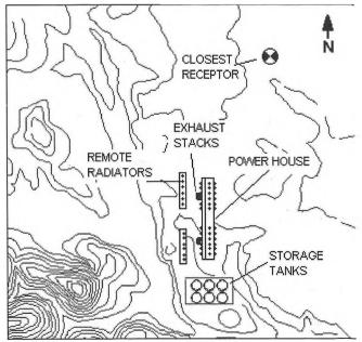
Figure 2: Plant Layout with Elevation Contours
