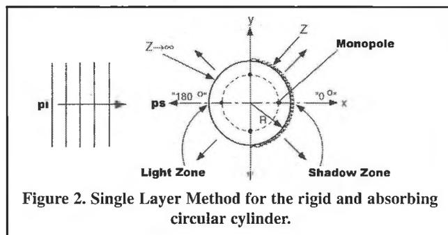
Figure 2. Single Layer Method for the rigid and absorbing circular cylinder.
