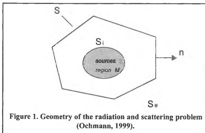
Figure 1. Geometry of the radiation and scattering problem (Ochmann, 1999).
