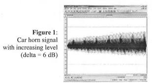
For listening conditions of the car horn in background noise, a 2-sec traffic noise recording was taken the CD library of environmental sounds. Using MATLAB, the bank of increasing and descending car horn signals was mixed with the constant traffic noise at a signal/noise ratio of + 6 dB.
