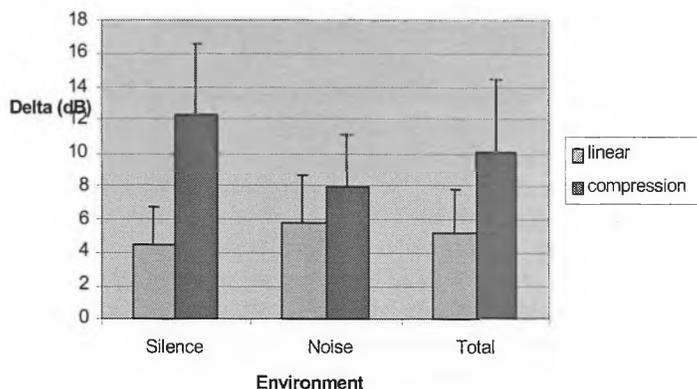
with a compression ratio of 3:1 made intensity changes 1.98 times more difficult to perceive than with a simulated linear hearing aid. This is illustrated in Figure 2.
