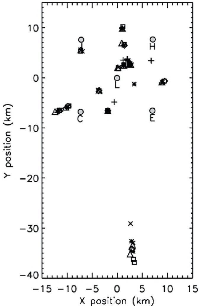
Fig. 1. 2002 results: Laurinolli and Hay (x); Simard *et al.*, spectrum coincidence(o); Simard *et al.*, cross-correlation(\*); Morrissey *et al.* (+); Simons *et al.* (◇); Desharnais *et al.* (Δ). Shaded circles indicate the OBH positions.
