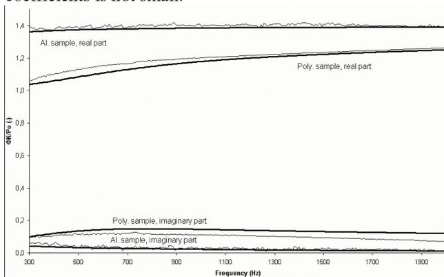
Fig. 2. Bulk modulus as a function of frequency for two real samples. Computed by Brownian motion simulations and compared to measurements for (i) identified (Duocel® al. foam 40 ppi) and (ii) scalded (polymeric foam) Kelvin structures. Top: real parts. Bottom: Imaginary parts.
