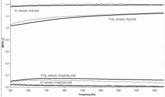
Fig. 2. Bulk modulus as a function of frequency for two real samples. Computed by Brownian motion simulations and compared to measurements for (i) identified (Duocel® al. foam 40 ppi) and (ii) scalded (polymeric foam) Kelvin structures. Top: real parts. Bottom: Imaginary parts.
