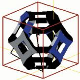
Fig. 1. The Kelvin structure paves periodically space. A "random walker" is seen. It serves to compute an essential thermal dissipation function, the dynamic bulk modulus.
