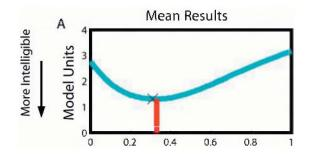
Fig. 1. The x-axis the gain in dB for every dB shift from an audiogram mimicking the NAL-R's gain ratio of 0.31. The X marks the NAL-R prescribed gain ratio, while the vertical bar is the Neurocompensator optimized value 0.32.
