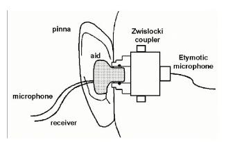
Fig. 2. Procedure for measurement of open-loop transfer function and ear canal sound pressure.
