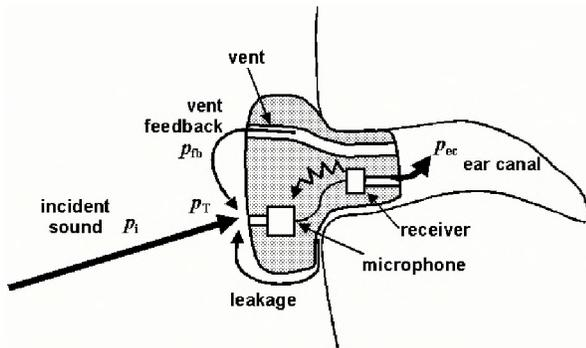
Fig. 1. Sketch of a hearing aid in an ear canal, showing several possible feedback paths.
