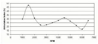
Fig. 4. Results of Articulation Index with respect to Engine Speed.
