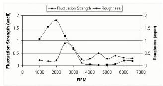
Fig. 3. Results of Fluctuation Strength and Roughness with respect to Engine Speed show very little low frequency and moderate mid frequency modulation of the induction noise data.
