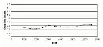
Fig. 2. Results of Sharpness versus Engine Speed show very little high frequency content in the induction noise signal.
