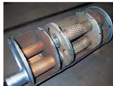
Fig. 1. Cutaway view of the muffler used showing the multiple passages and chambers that make up this reactive filter.
