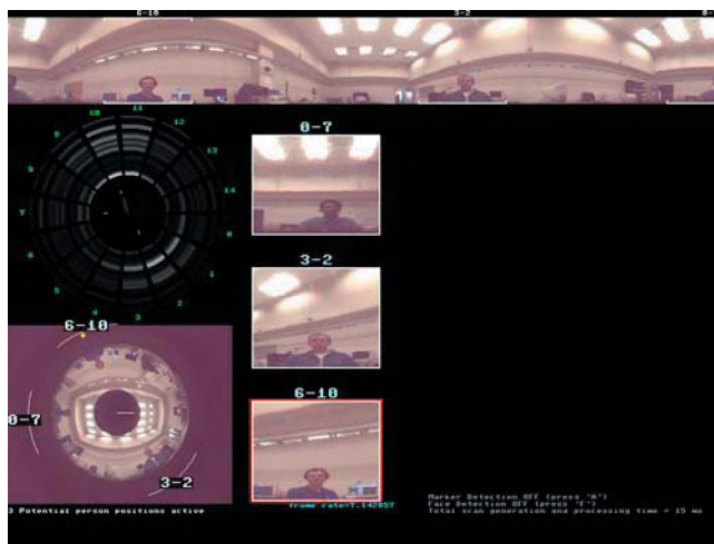
Fig. 2. Panocam. The raw video image appears in the lower left. The initial corrected panoramic image appears at the top. The real-time audio search response shows an active talker near 12:00 in the left centre frame and three virtual images are shown in the centre frame. The audio and corresponding virtual video (lower image, "6-10") is selected for output.
