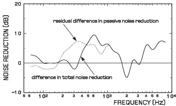
Figure 1: Difference between passive, and total, noise reduction
