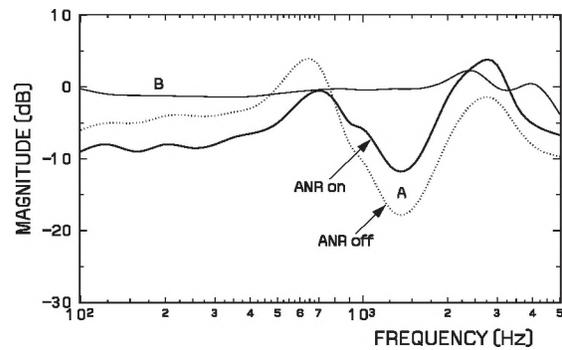
Figure 2: Frequency response of sound reproduction sub-systems
