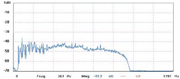
Figure 2. Spectrum from figure 1 with hum reduced using a comb filter.
