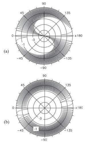
Fig. 3. Polar plots of the envelope of the beam-patterns for the bent array. Steering angles are relative to (a) the *x*-axis and (b) the regression axis. Beam peaks are at 0 dB and rings at -1-dB intervals.
