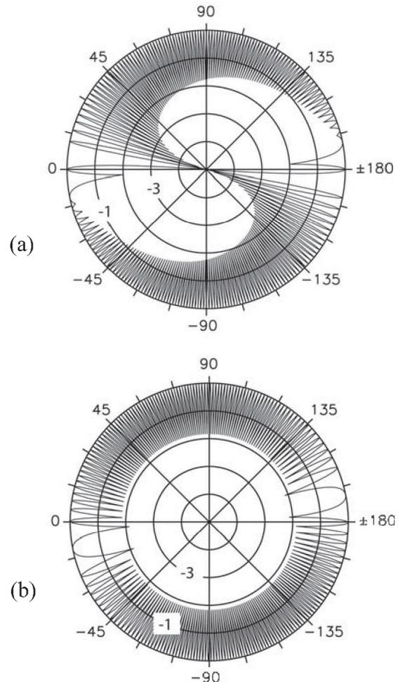
Fig. 3. Polar plots of the envelope of the beam-patterns for the bent array. Steering angles are relative to (a) the  $x$ -axis and (b) the regression axis. Beam peaks are at 0 dB and rings at  $-1$ -dB intervals.
