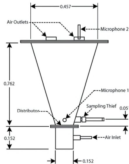
Fig. 1. The fluidized-bed dryer dimensions in meters.
