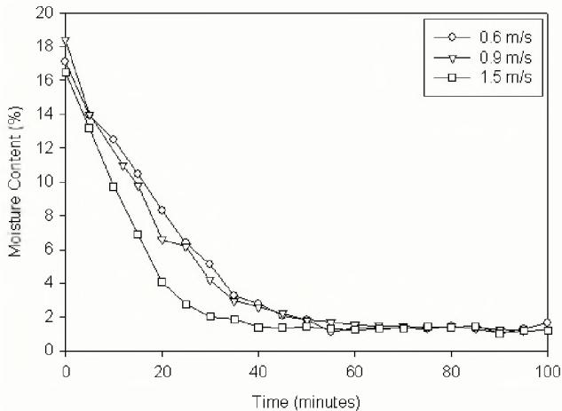
Fig. 2. Moisture content of granule samples taken during the drying process.
