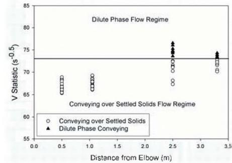
Fig. 3. V Statistic values for polyethylene pellets from the wavelet residual acoustic signal for all distances from the elbow, identifying the two flow regimes.
