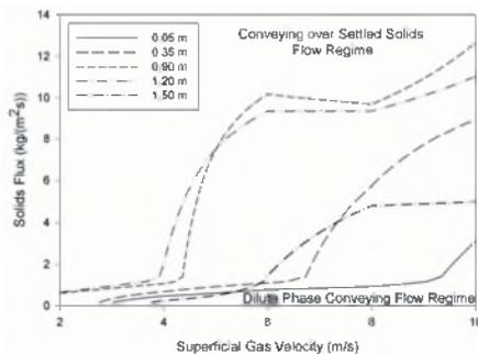
Fig. 2. Flow regime map for glass beads at various distances from the elbow.
