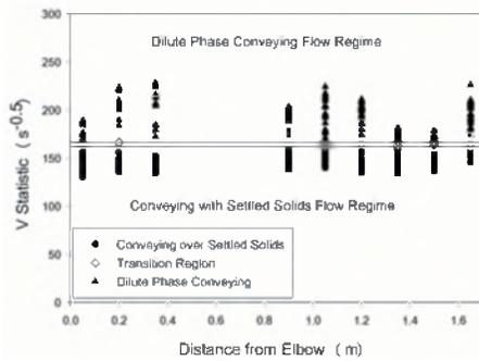
Fig. 1. V Statistic values for glass beads using wavelet residual of acoustic signals for all distances from the elbow, identifying two main flow regimes and narrow transition region.
