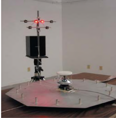
Figure 2 System setup. The 16-microphone array, panoramic camera (center of array), speaker on tripod, and LED light system are shown. Another speaker and light system are located 120° about the array.
