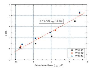
Fig. 2 Value of k versus reverberant level in the receiving space.
