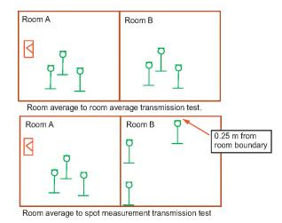
Fig. 1 Conventional room-average to room-average measurement approach (upper) and the new roomaverage to spot-receiver position approach (lower). Using equation (2) and an estimate of k from Fig 2, one can predict received sound levels,  $L_{0.25}(f)$ . Fig. 3 compares measured and predicted  $L_{0.25}(f)$  for the three test walls. For the speech frequency range from 160 to 5,000 Hz, the average differences between measured and predicted  $L_{0.25}(f)$  were 0.24, 0.17 and -0.19 dB.
