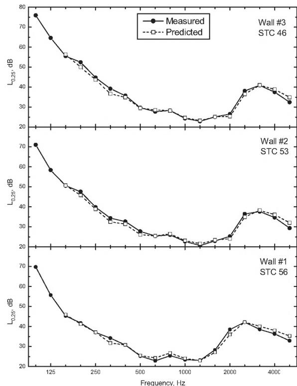
Fig. 3 Comparison of measured and predicted  $L_{0.25}$
