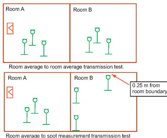
Fig. 1 Conventional room-average to room-average measurement approach (upper) and the new room-average to spot-receiver position approach (lower).
