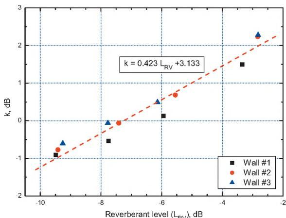
Fig. 2 Value of  $k$  versus reverberant level in the receiving space.
