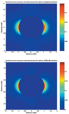
Fig. 1. Analytical (top) and FEMLAB (bottom) solution for the elastic scattering problem. The plots show the near-field pressure intensity for a slice parallel to the direction of wave propagation (left to right) through the origin. The solution inside the sphere was not calculated.
