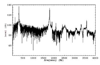
Figure 3: Spectrum of note D3. Notice the fundamental at 304 Hz, the first overtone at 1780 Hz, and a second overtone at 3560 Hz (highly attenuated).
