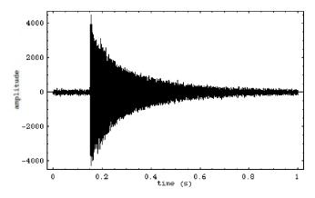
Figure 2: Waveform of note D3. Notice the sharp attack and exponential decay of the waveform.
