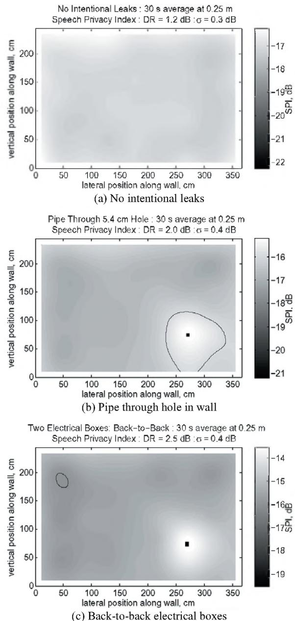
Fig. 3. *SPI* at 0.25 m from the wall, calculated for 65.7 dBA speech and 31.5 dBA noise. The contour is for -16 dB, which corresponds to the threshold of intelligibility. All plots self-normalized so that lightest grey corresponds to peak *SPI*.
