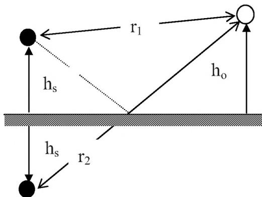
Figure 1. Simple source above a reflecting plane
