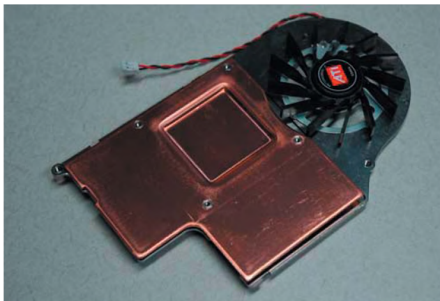
Figure 2. Disassembled Fan and Mounting Tray.
