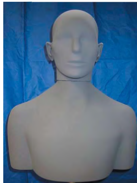
Figure 4. Binaural Head Manikin used Acoustic Data Acquisition.
