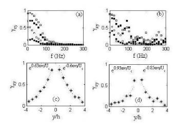
Fig. 2. Coherence spectrum of surface pressures obtained (a) experimentally and (b) numerically between the center reference point (y/h=0) and two other transverse locations: y/h~-0.5 (□:uniform; ■: notched), y/h~-2.08(○:uniform;
