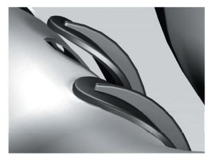
Fig. 2. Experimental tonehole design without chimney.
