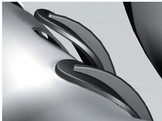
Fig. 2. Experimental tonehole design without chimney.
