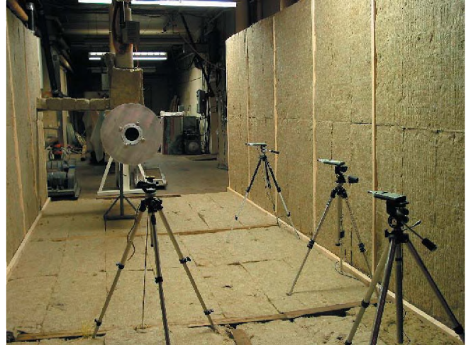
Figure 2. Cabin outflow valve noise measurement
