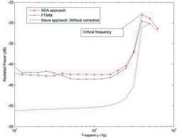
Fig.2. Radiated power of a single plate excited by a random force.
