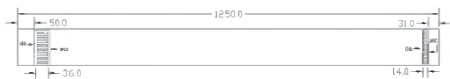
Fig. 2. Sketch of the heat driven thermoacoustic refrigerator with helium, all dimensions are in millimeters
