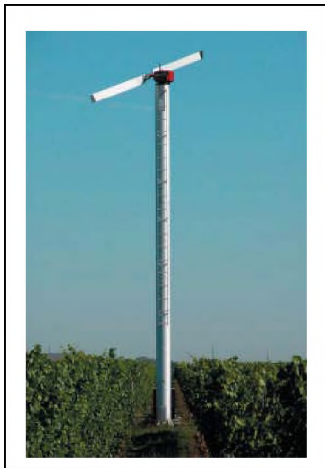
Figure 1: Typical wind machine in a vineyard
