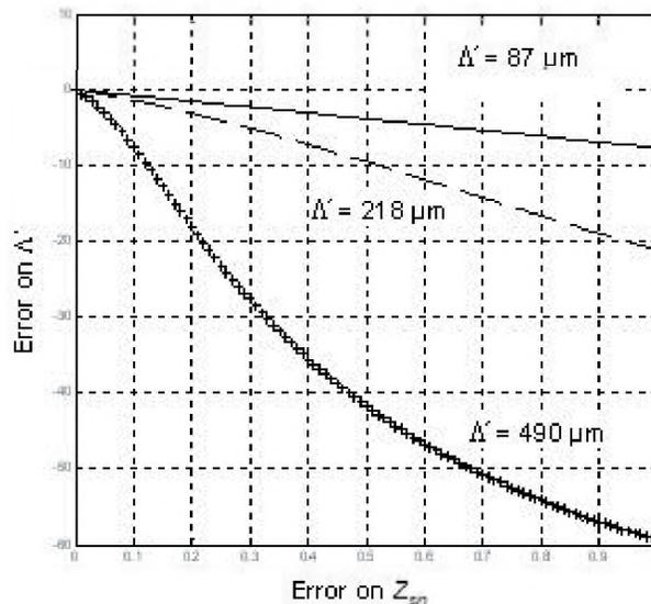
**Figure 1 : Error on inversely found  $\Lambda'$  in function of the error on  $Z_{sn}$**
