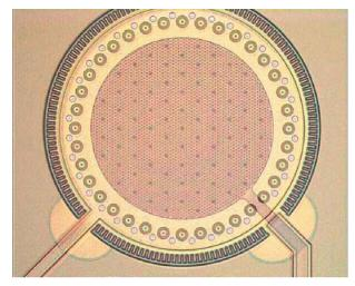
Fig. 2. SiSonic MEMS microphone diaphragm [1].
