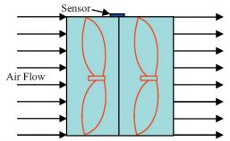
Fig. 6. Double fan configuration with an acoustic pressure sensor placed at the mid point of the two fans.
